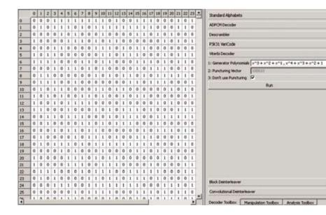
By including and using the generator polynomials in the Viterbi decoder, the convolutional coding on the bit stream is reversed.
